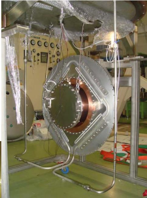
300kW 1kHz phase shifter tested at SP8
