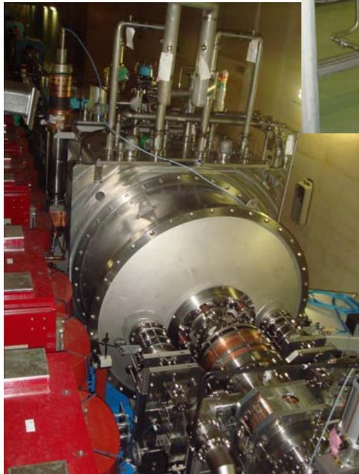
Crab cavity installed to KEK-B (Jan. 2007)
